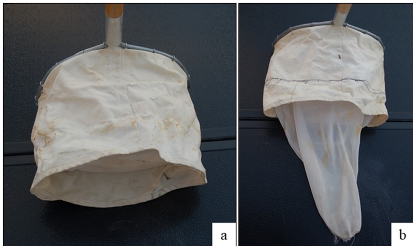
Figure 2 Collection nets discussed in this manuscript. a – a standard, commercially available, truncated D-frame net with 500 µm mesh; b – our custom made, non-truncated D-frame net with 250 µm mesh.
