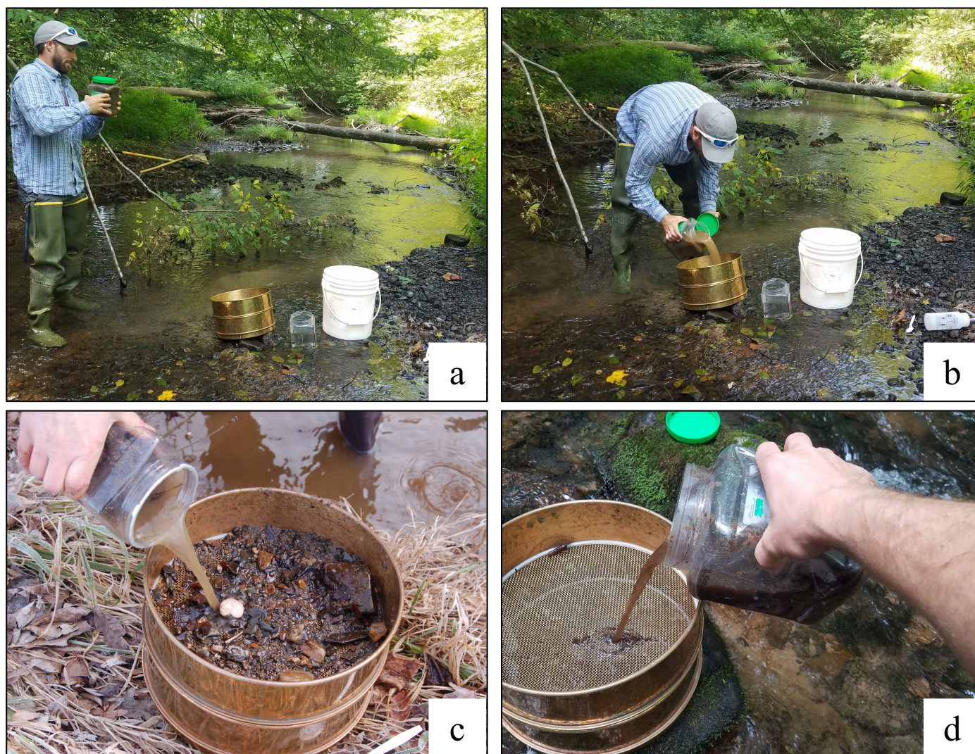
Figure 6 The sieving process proposed in this manuscript. a – collector fills the composited sample container with water and shakes the container for approximately 10 seconds; b – immediately after shaking the collector removes the lid and pours the water through the 3mm and 250 µm sieves; c and d – the 3mm will be placed on top of the 250 µm sieve so it can filter out larger sized substrate and debris. This process is repeated 10x.
