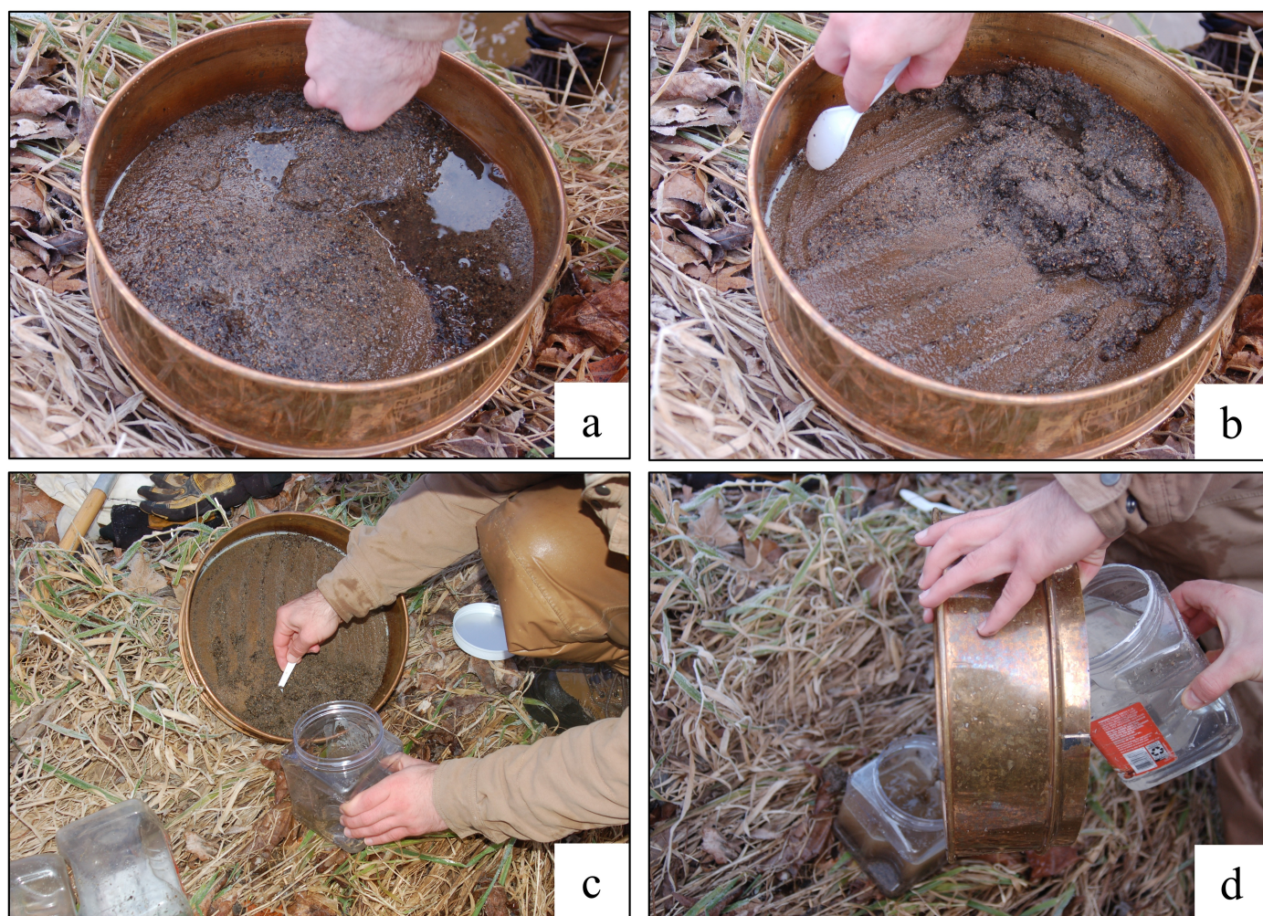
Figure 7 After sieving, the collector removes the contents from the 250 µm sieve and places them into the final sample jar. a – fine sediment and water mites accumulate in the 250 µm sieve; b – using a plastic spoon or similar tool, the collector can scrape the sediment to one side of the sieve; c – the contents of the sieve are removed and placed in the sample container; d – once the contents from the sieve have been removed, the collector can tilt the sieve vertically above the sample container and using a separate, clean container filled with stream water, the collector can slowly pour the water through the back of the sieve to rinse any remaining sediment and water mites into the final sample container.
